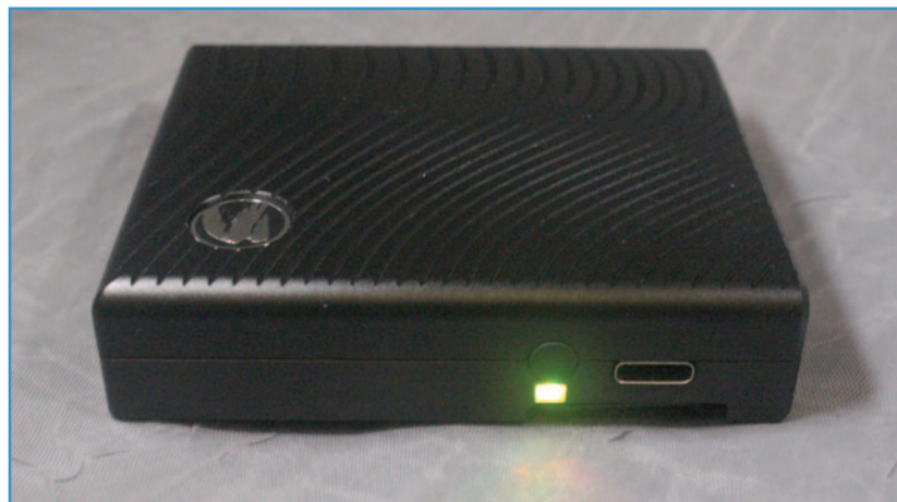
Ruby side view with power switch, LED, and USB port.
