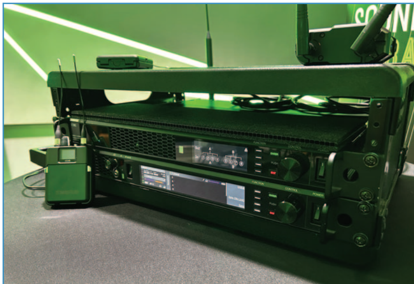
The ADXR body-pack receiver, AD8C eight-port antenna combiner, and ADTQ wireless quad transmitter.
