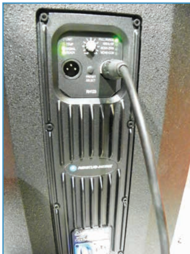
LEDs on the amp module indicate ready, signal, temperature, and limit.
