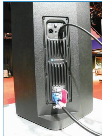
Power to the amplifier is via Neutrik Powercon, with a looping output for daisy-chaining additional speakers.
