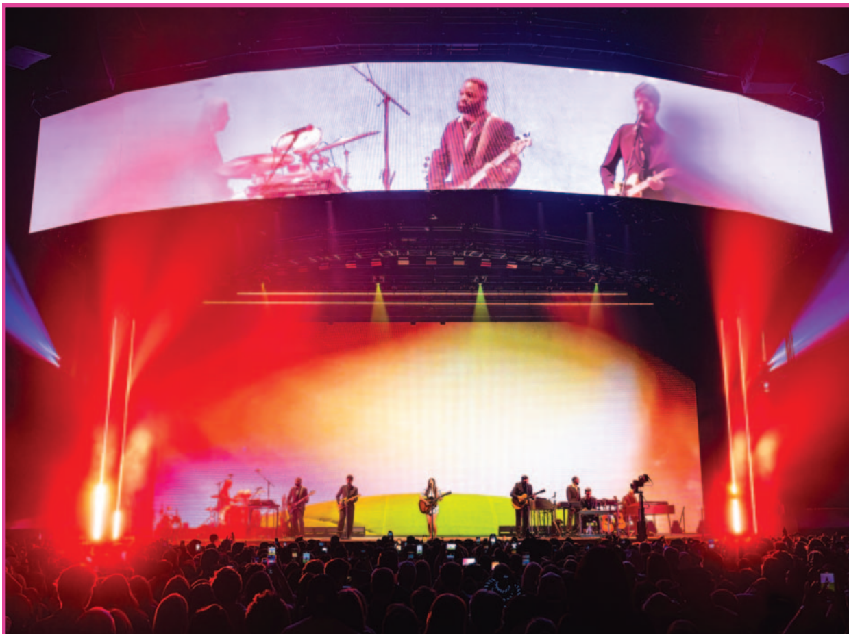
Imagery is seen on a combination of ROE Visual solid and see-through screens with Barco UDX-4K 40K projectors pointed at the stage and additional 40Ks for the side screens. Upstage are Vanish V8Ts in a configuration 23m wide by 9m tall). The eyebrow features ROE CB5s, in a configuration 25.2m wide by 3.51m tall.
