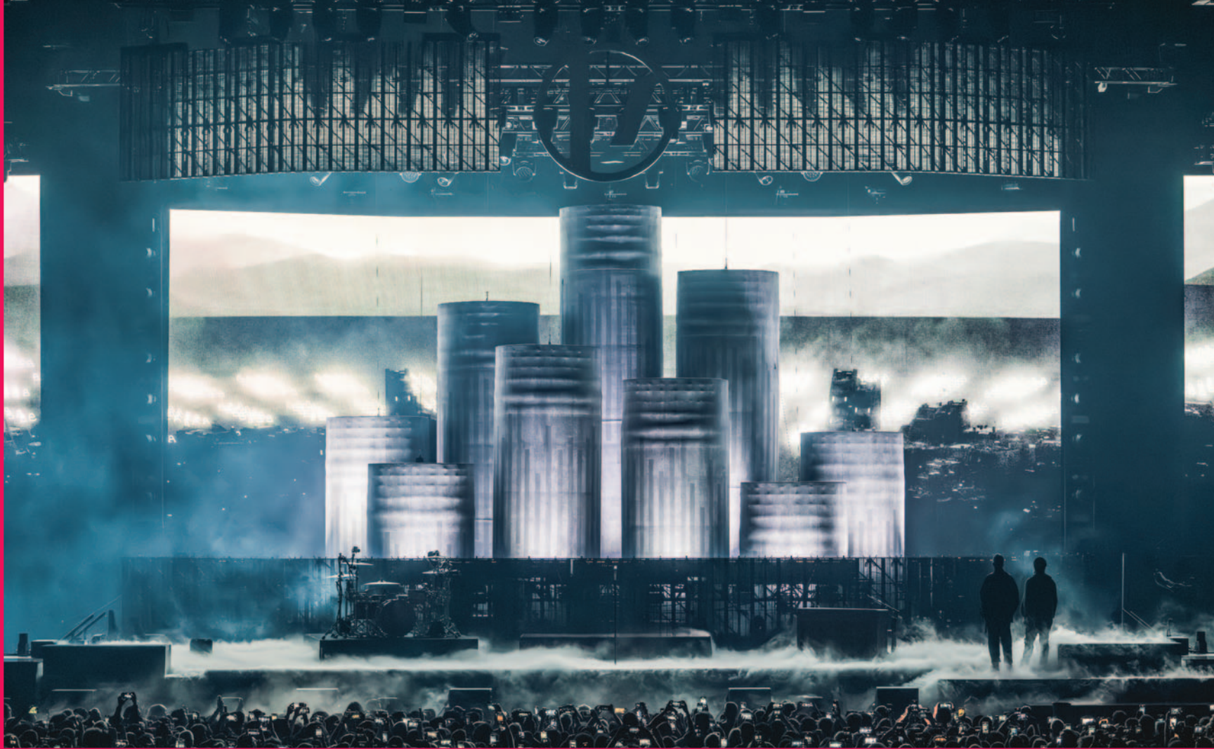
The video walls consist of SACO 9mm panels, supplied by Nighthawk Video. The prerendered media and real-time effects are handled on the Disguise media server, which can be programmed to run with time code or triggered on the fly.
